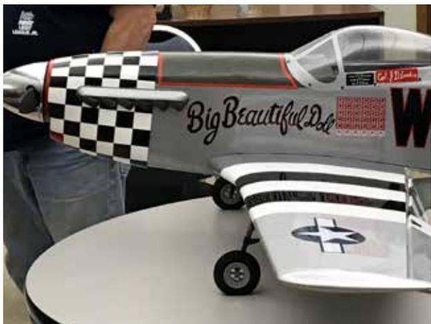
Gary Keup brought in a World Models P-51 he is repairing. It is a rebuild he got from a former member, Aaron Cochrane. He has modified it for retracts, and is thinking about a DA-50 for power. It has an 82" wingspan, with final weight to be determined. He is sourcing parts from Great Planes including the cowl, canopy, and decals.
