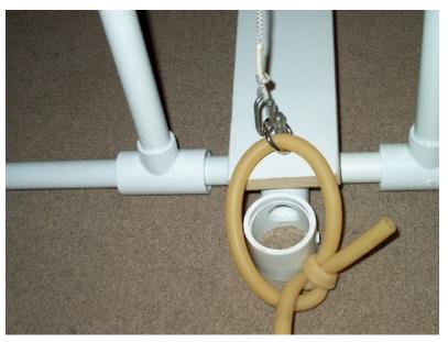
**Pictured above:** The releasing pin holds at one end the taut portion of surgical tubing. At the opposite end of the pin is a nylon chord that is taut to the airplane which is in a ready to launch position. The nylon chord easily attaches to a hook on the plane. Once the foot pedal is pushed the see-saw plate pivots above the releasing pin's height allowing the taut surgical tubing to pull or launch the plane into flight.
